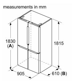
A: Front is adjustable from 1830 to 1847, with front levelling feet fully extendedB: Add 25 for fixed spacers on back
