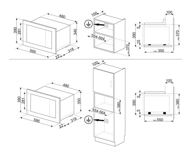
PLEASE NOTE: not designed for under bench installation. PLEASE NOTE: drawings are not to scale. They are to assist only. WARNING: technical specifications and product sizes can be varied by the manufacturer without notice. Cutouts for appliances should only be by physical product measurements. The above information is indicative only.
