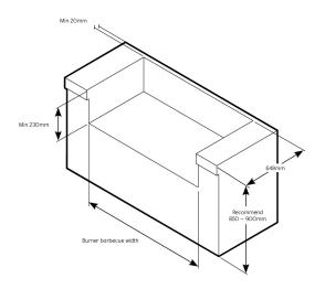
For built-in installations: islands, masonry, other non-combustible material structures.
