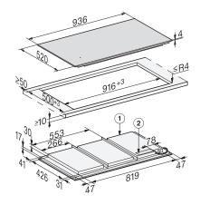
1.Front. 2. Main connection box (The mains connection cable (L = 1,440 mm) is supplied loose)
